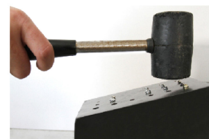
■ 头部敲击实验 Screw head hitting test
